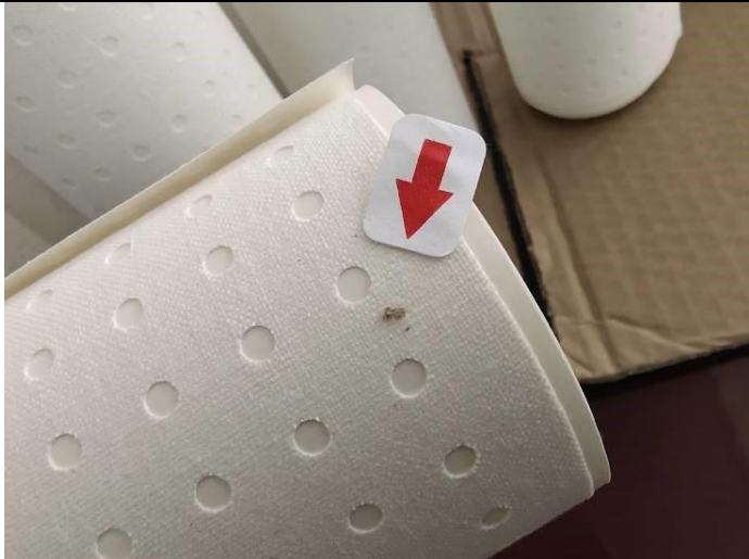
Dirty mark on surface -minor
