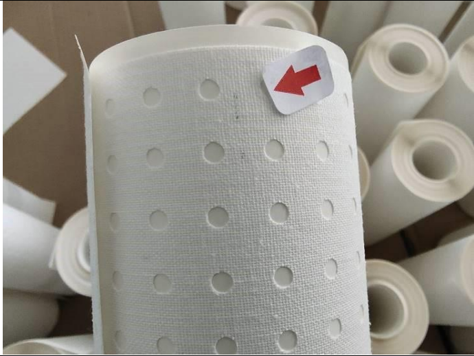
Dirty mark on surface -minor
