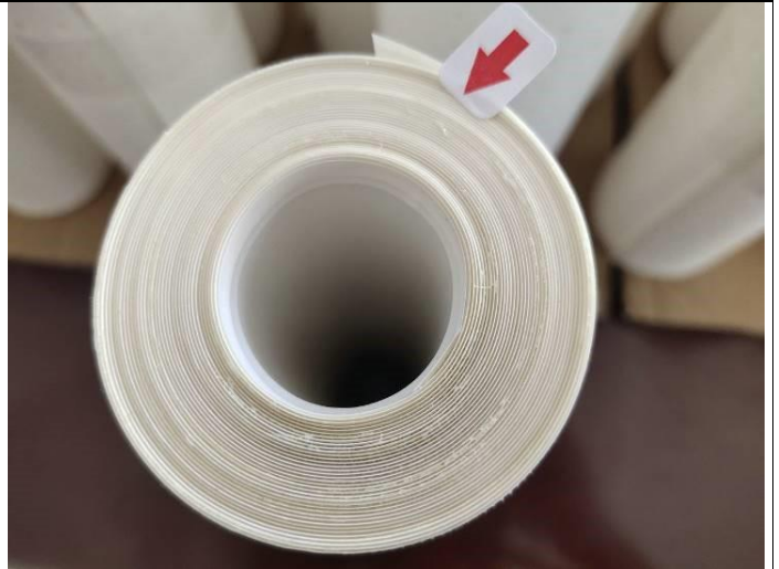
Glue mark on surface -minor
