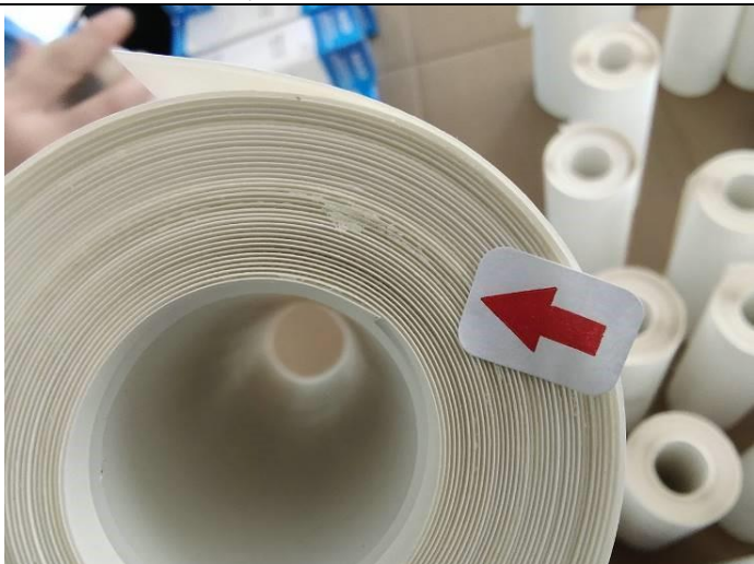
Glue mark on surface -minor
