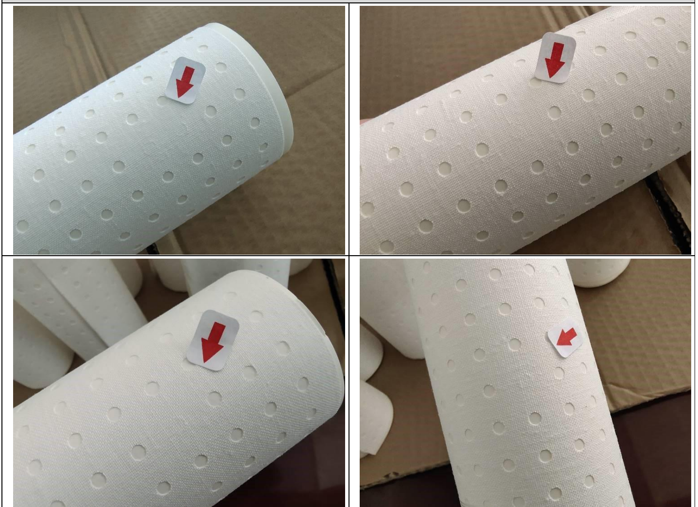
Remark 2: Actually found a small amount of no punching holes on product surface, 100% of sampled products have this problem.
