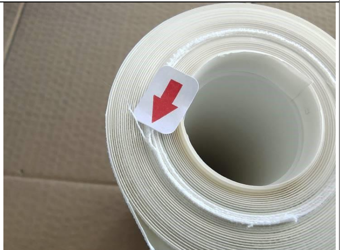
Untrimmed thread end-minor
