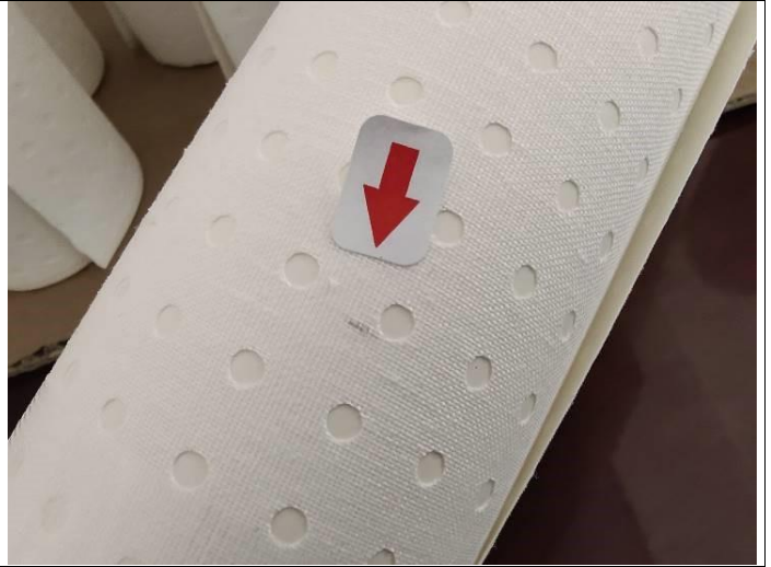
Dirty mark on surface -minor
